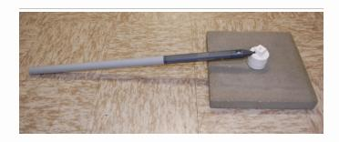
A **quick-change mount** is a convenient option for deploying tilt current meters without having to remove a meter's lanyard from the anchor itself. You will need some PVC fittings and materials typically found in hardware stores. For detailed instructions download our Quick-Change Mount Application Note here: <u>QUICK-CHANGE MOUNT</u>
